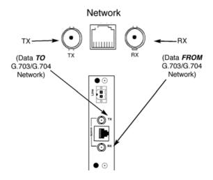
Figure 6. 75 ohm Dual Coaxial G.703 Interface
